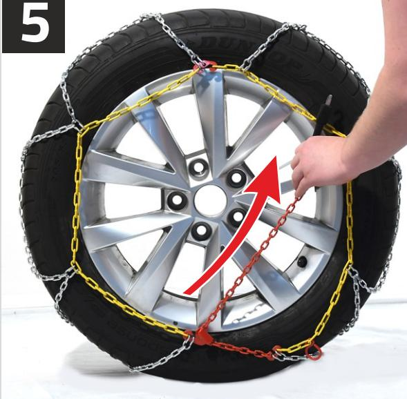
Put the fixing chain into the slot slide hook so that the eyes of the chain fit into the free slot in the hook. Fixing chain pass through the eye of the side chain.
