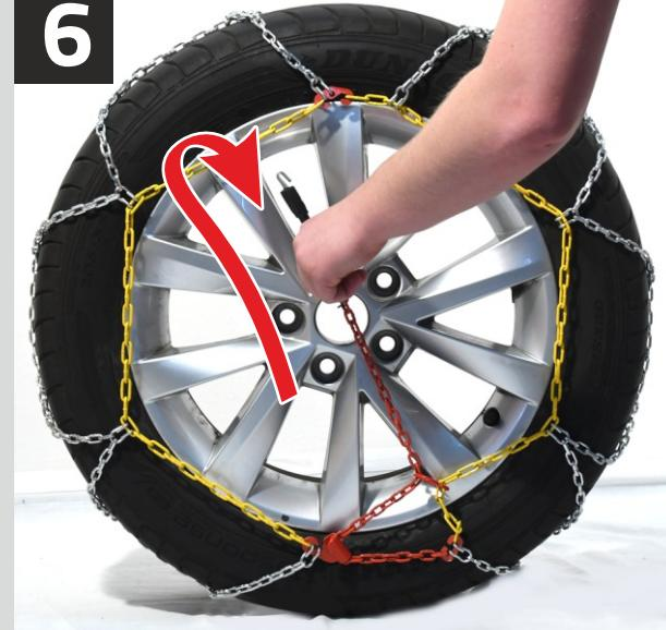
Tight the fixing chain and fix the rubber hook to secure eye on the side chain. After driving 50 meters check show chain position. If necessary, retighten. While driving, check the consolidation periodically!
