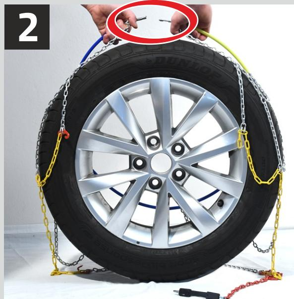
Join the circuit rope on the top side of the wheel.
